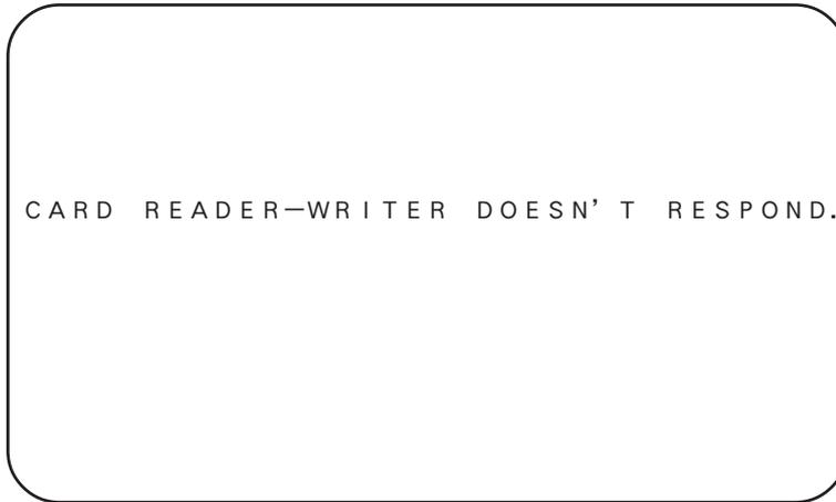
FIG. 7 e CARD READER/WRITER CONNECTION ERROR Screen
