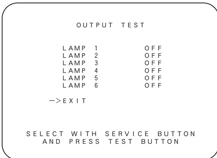
Selecting OUTPUT TEST displays the following screen and allows the status of each lamp to be checked.
