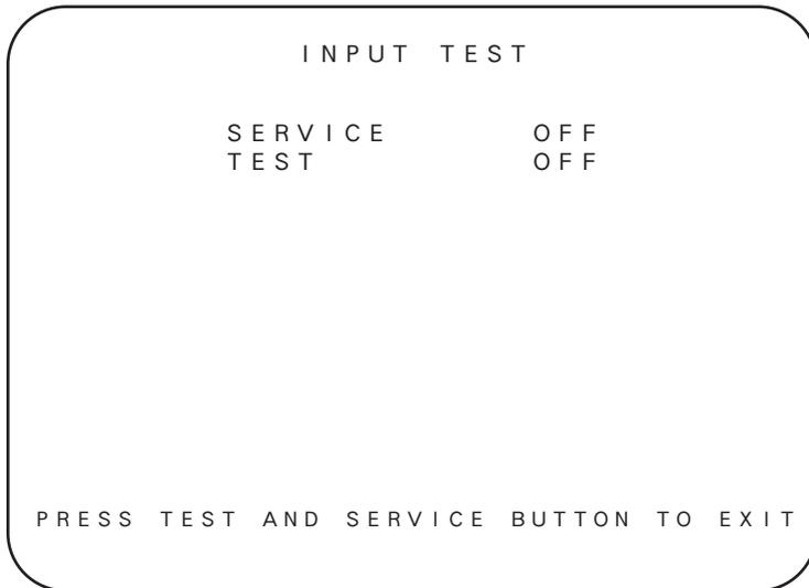
Selecting INPUT TEST displays the following screen and allows the status of each input device to be checked.
