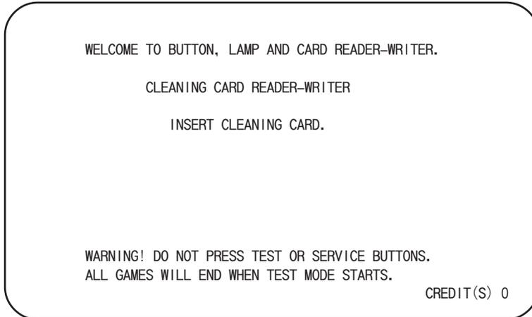
Select **CLEANING CARD READER-WRITER** and the display will switch to the following screen, allowing you to clean the head of the card reader/writer.
